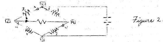
In figure 2, x, y, z, u, and w are currents measured in the directions shown by the arrows. The numbers by the  $\$  WW symbol represent the size of the resistance in ohms. The numbers in the boxes (10, 0, p, q) represent the potentials at each junction in volts. Using Ohm's Law we have 5 equations:
